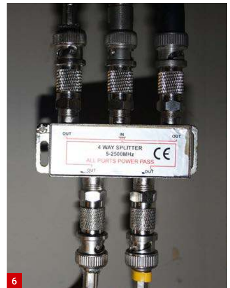
Fig. 2: A VNA sweep, demonstrating insertion loss of a four-Port splitter. Fig. 3: Typical four-port isolation. Fig. 4: Some typical impedance and VSWR measurements of an output port. Fig. 5: Top: Isolation measurement; bottom: insertion loss of an eight-port splitter. Fig. 6: A four-way splitter in use with BNC-to-F adaptors.
