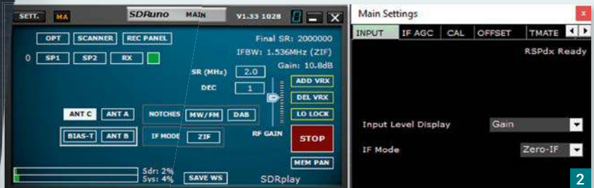
Fig. 1: The RSPdx being shown at the start of the Nevada and Waters & Stanton Open Day. Fig. 2: The SDRuno main panel for an RSPdx includes a choice from three software-selectable antenna inputs. Fig. 3: The SDRuno RX Control Window now has new 'HDR' band buttons for the sub-2MHz frequency bands. Fig. 4: A comparison table, showing where the RSPdx fits in the SDRplay products range. Fig. 5: A screenshot of the RSPdx receiving clean long wave signals (from SDRplay's introductory video). Fig. 6: A screenshot from Mile Kokotov's YouTube video showing the RSPdx at 40m. Fig. 7: A screenshot from Oxford Shortwave: a transatlantic MW signal from WFME New York using HDR mode.
