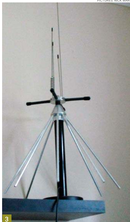
Fig. 1: Nick's Sangean DAR-101VOX recorder. Fig. 2: Nick's current meteor monitoring station. Fig. 3: Nick's discone aerial on a shelf.
